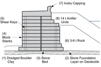
Figure 29—Construction Sequence
