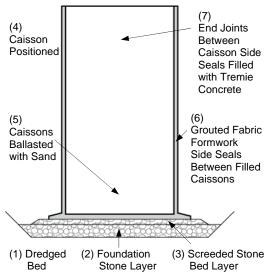
Figure 13 – Construction Sequence
