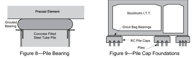
Structural piles or shafts can be used to support precast elements although this is not common. Grouted top bearings can be used to large diameter piles. Alternately pile caps can be cast to pile groups and grouted fabric formwork or other bearings cast after the element is positioned. Precast pile cap shells are often used in America to form pile caps around water level.
