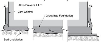
of negative buoyancy of the element and reduces size of temporary the support jacks and/or foundations. Formwork systems are designed to cope with foundation tolerances, excavation grouting withstand pressures, control uplift forces and give good base contact and reliability.
