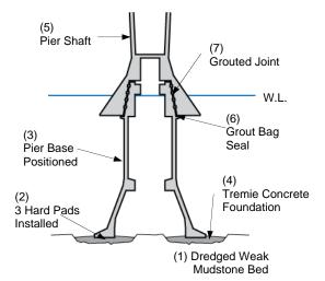
Figure 23 – Construction Sequence
