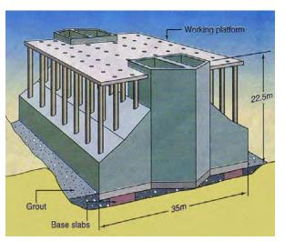
Figure 6 \*—Grout Washout, Oresund Bridge Pier
