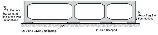
Figure 24—Construction Sequence
